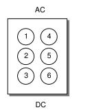
AC/DC switch viewed from behind (pins facing toward you). With switch in the up position (AC) pins 2 and 3 are connected, and pins 5 and 6 are also connected.
