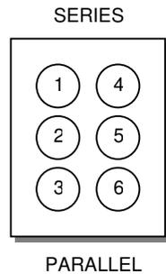
Switch viewed from behind (pins facing toward you). With switch in the up position (SERIES) pins 2 and 3 are connected, and pins 5 and 6 are also connected.
