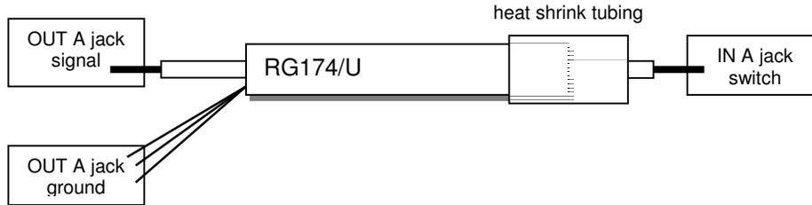
SW1 is connected to the PCB with four pieces of coax cable. Pads on the PCB (S1, S2, S4, S5) indicate which of the four switch pins to connect using the following numbering convention:
