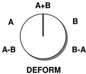
When normalled to the Tank A and Tank B amplifier/resonator outputs, the A-B and B-A deformations have the ability to cancel significant portions of the input signal while leaving much of the reverb signal untouched<sup>6</sup>.
