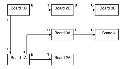
Future versions of the MUUB boards will have larger holes specifically for chaining power supply connections between boards.
