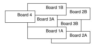
Boards 2B, 3B, and 2A are on the first layer, nearest the Stooge "flat plate modular bracket". Boards 1B, 3A, and 1A are on the second layer (mounted above the first layer). Board 4 is mounted above board 3A on the third layer.
