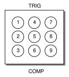
Switch viewed from behind (pins facing toward you). With switch in the up position (Trigger Mode) pins 2 and 3 are connected, pins 5 and 6 are connected, and pins 8 and 9 are connected.
